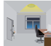
With sufficient natural light,the sensor switches on the light automatically when person enters the room
