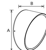
NL65D LED bulkhead which adopts high lumen 2835 SMD light source, PC diffuser and ADC12 aluminum. It has a high transmittance and uniform light output. High protection level IK10&IP65, high lumen efficiency 100lm/W with 110° beam angel are available. More functions: CCT interchangeable, triac dim wth flicker free and S7 sensor.
