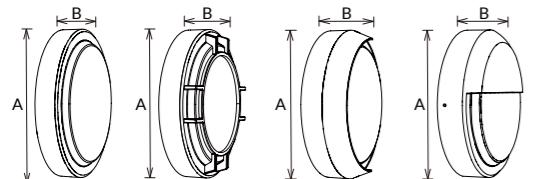
NL104 is IP65 IK10 bulkhead which adopts Die-casting Aluminum body and 94-V0 fire-rated PC cover. This fixture is with four different trims and provides an alternative to color changeable, sensor and emergency functions. Dali and 0-10V dimming is also available.
