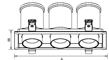
ND297A LED downlight adopts high lumen COB light source, the special optic lens and reflector design offer a uniform light output and low glare effect. It is an extension design, 360 degree horizontal rotation and 68 degree vertically rotation. And it has round shape, square shape with single/triple heads which is suitable for various application area.
