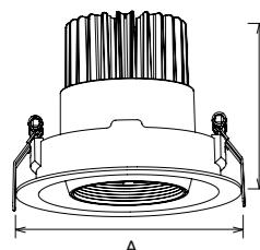
ND122 Gimbal downlight adopts brand CITIZEN COB, exchangeable reflector and tempered glass, ADC12 aluminum heatsink. Horizontally 355° and vertically 30° rotatable. External driver is exchangeable through quick connector among non-dimmable driver, Triac dimmable, 0-10V and DALI dimmable drivers.
