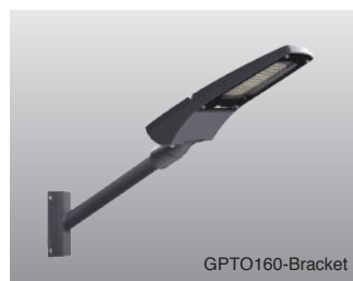
Wall bracket in 50-cm length with boom diameter of 60mm and 30 degrees angle
